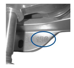
THIS NUMBER IS REFERRED TO THE DISTANCE (EXPRESSED IN MILLIMETERS) BETWEEN THE CENTER OF THE AXLES. BUT IT'S IMPORTANT TO NOTE THAT THE NOMINAL SIZE IS NOT INDICATING THE TOTAL LENGTH OF PLATE.
